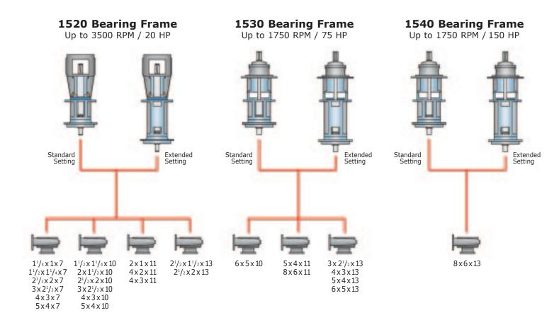
The simple design of the GVC is augmented by its modular construction. All twenty-five sizes are based on only three bearing frames and share most of the same parts as our other industrial product lines.
